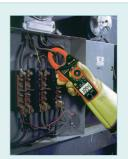
True RMS meter gives you accurate readings of non-sinusoidal waveforms
