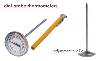
These pocket-sized dial thermometers feature either a  $\varnothing 25$  mm or  $\varnothing 45$  mm dial with a pointed  $\varnothing 4$  x 130 mm stainless steel stem and are supplied with a probe cover. Each dial thermometer is available in three scales. A stainless steel mounting clip is available.
