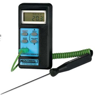
Seven models are available that utilise type K, J, T, R, N, S or E thermocouple probes. The instrument also features an auto-power off facility which maximises the battery life, turning the instrument off automatically after 30 minutes. Other selectable parameters include: display contrast and internal CJC temperature reading. For details of the extensive range of thermocouple probes available, see pages 49 to 54.
