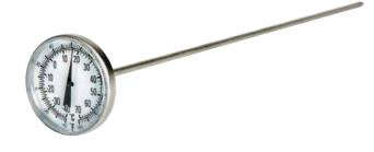
This simple to use  $\emptyset 45$  mm dial probe thermometer is reliable and accurate. The hot water dial thermometer features a  $\emptyset 4 \times 300$  mm pointed stainless steel stem. The thermometer indicates temperature over the range of -40 to 70 °C in 2 °C divisions.
